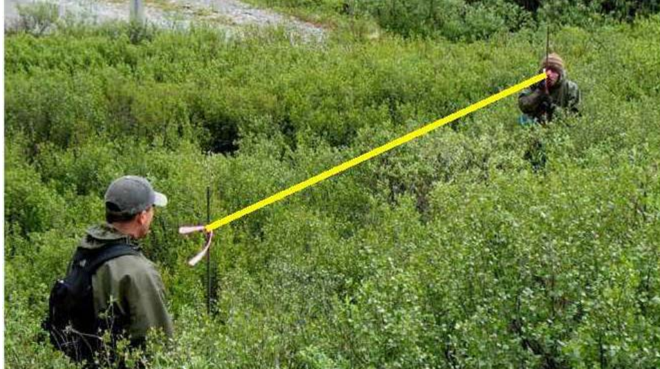
Photo 5.38 - Using Rebar to Mark a Horizontal Reference Point
